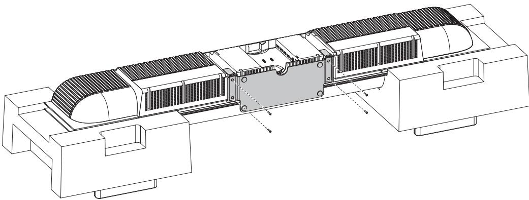
**UK:** Fasten with the four screws **② 2B**.
