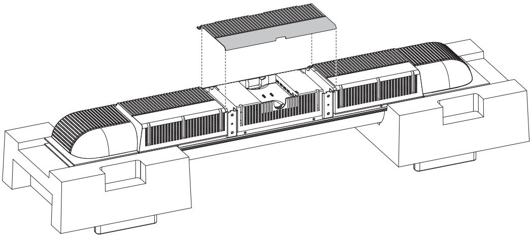
**UK:** Remove the connector cover from the central section by pulling gently.
