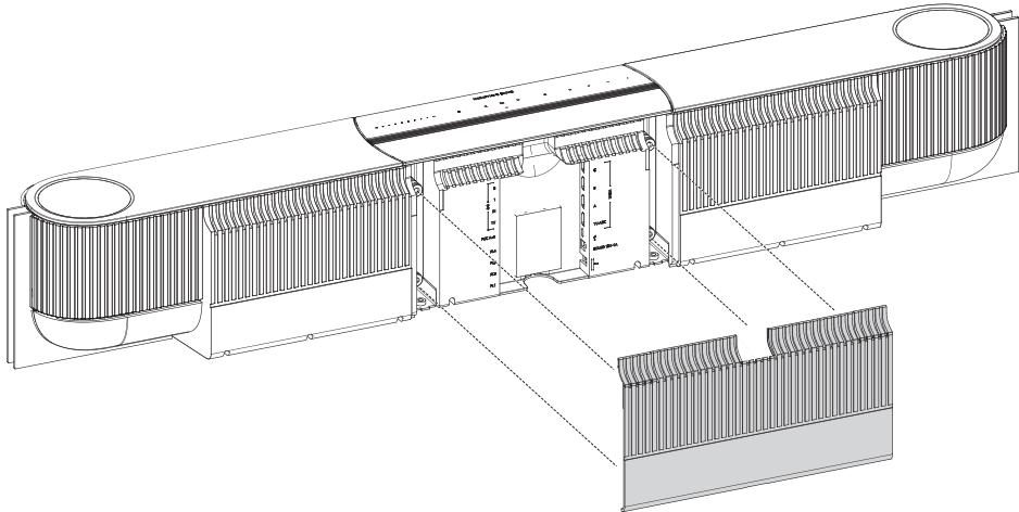
**UK:** Click the connector cover back on. Place the Soundbar at the desired location.
