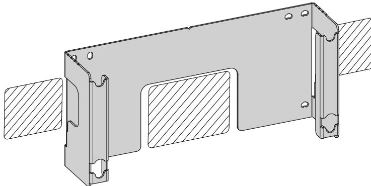
**UK:** Connect the relevant cables (see Appendix) and fasten them with the hook & loop fasteners. Cables can easily be routed in any direction on the wall bracket.
