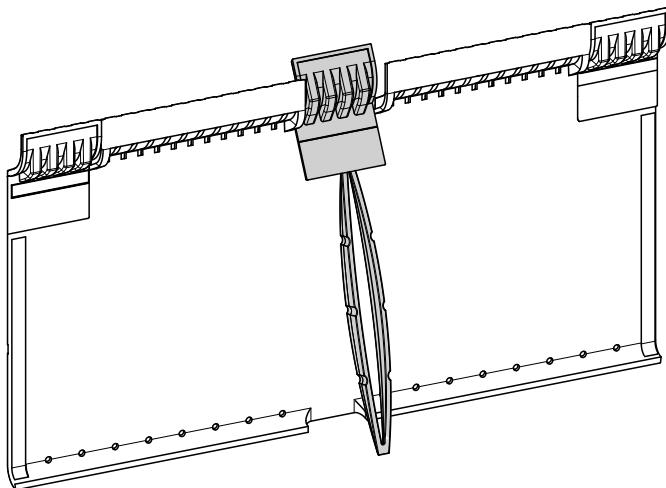
**UK:** Connect relevant cables in the connection panel (see Appendix). If you are installing the Soundbar under a TV screen, remove the detachable section in the middle of the cover so the cables can be routed upwards.
