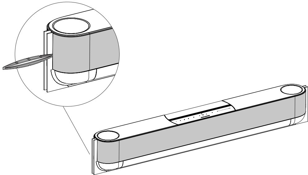
**UK: NOTE:** Use the tool in microphone box **6A** to remove the front cover. Start at the sides and work your way around, then pull at the top and bottom to remove the cover completely.
