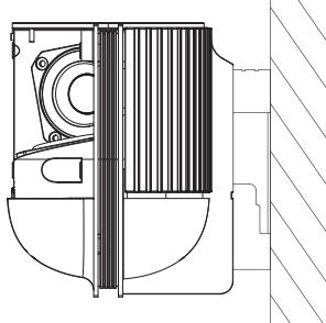
**UK:** Once it is cabled, hang the Soundbar on the wall mount. It can be placed in different positions. Make sure it is securely in the grooves, at your chosen depth. Make sure the cables aren't clamped or compressed. You can always make room for additional cabling by moving the Soundbar to the outermost groove in the installation spacers. Go to Step 3.
