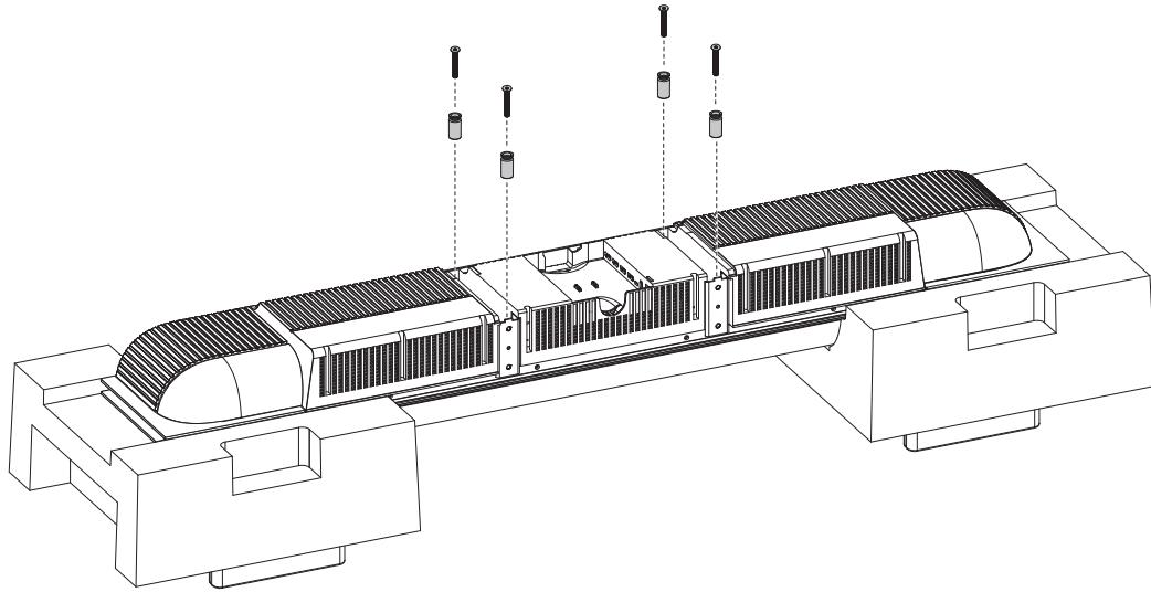
**UK: On the Soundbar:** Locate the grooved cylinders in the four corners next to the Soundbar's connection panel. Mount the four installation spacers (1) 2A on each, using the supplied screws (2) 2A.
