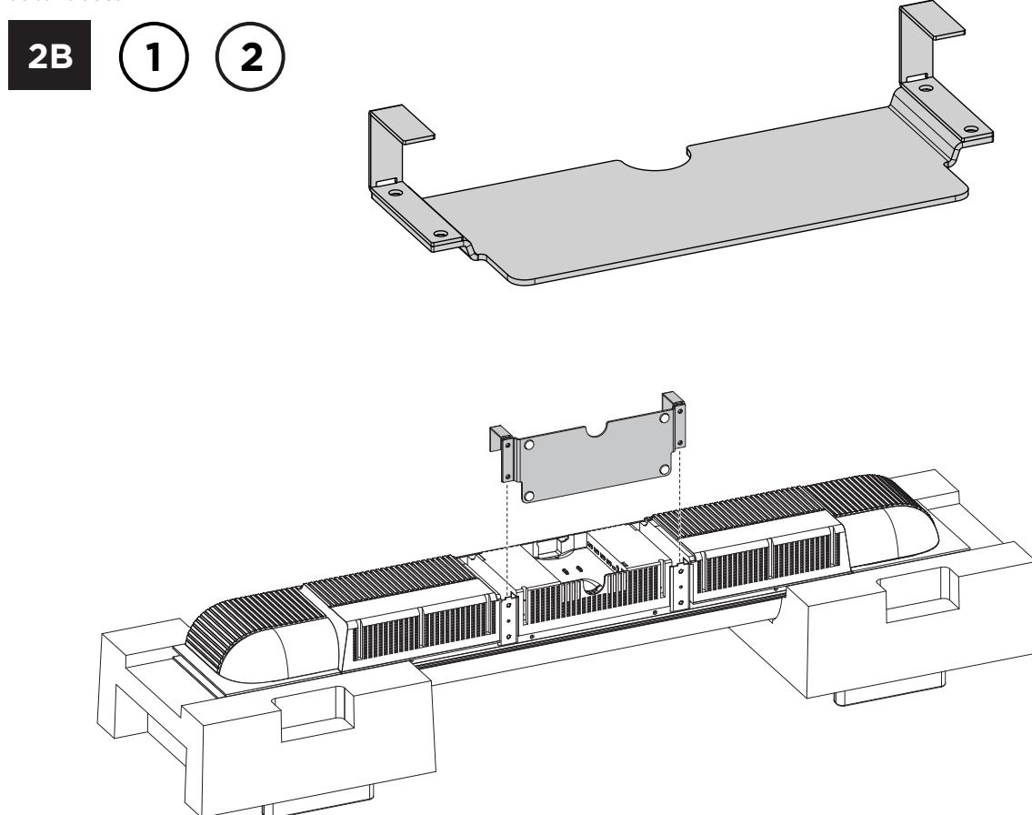
**UK:** Slide the Soundbar stand **① 2B** over the two lower cylinders next to the connection panel.
