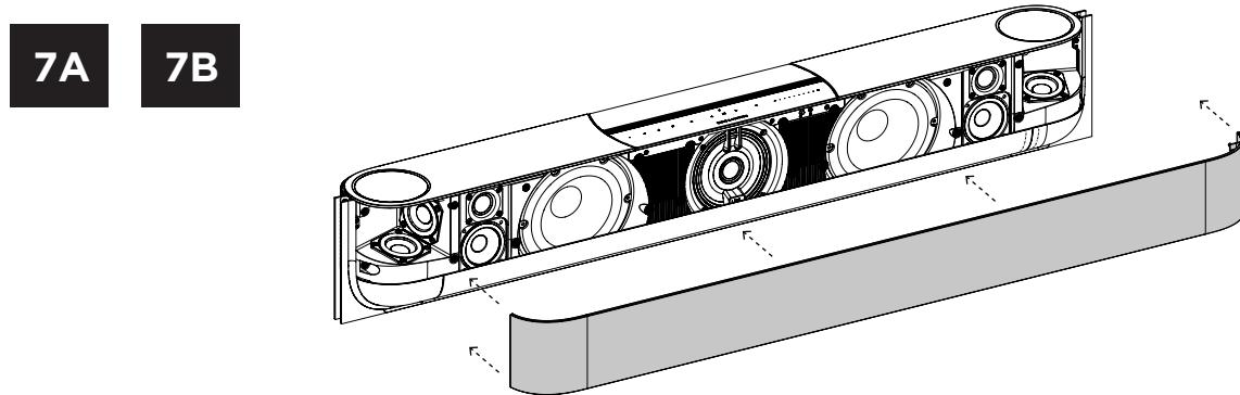
**UK: ON:** Locate the arrow on the front cover that shows you which way is up. Align the front cover pins with the sockets and push till the cover sits securely in position. Start at the centre then push the sides in. **NOTE:** Do not force the cover. If handled incorrectly, you risk breaking tabs or lamellas.
