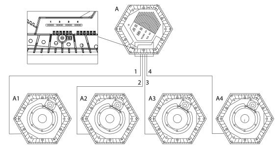
How to shorten the signal cables for the speakers
