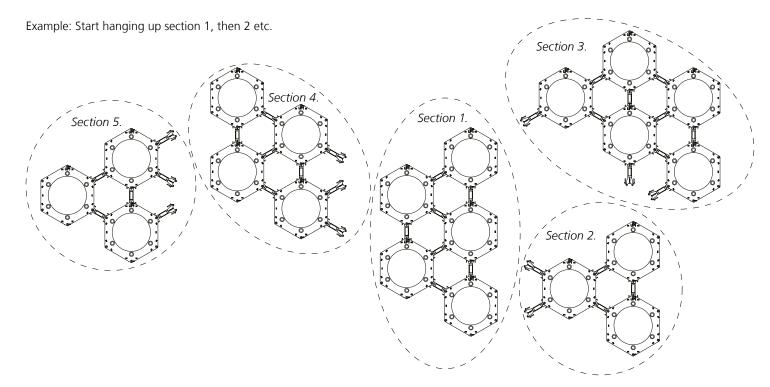
Disconnect the setup into smaller sections, e.g. 3-5 tiles depending on the setup. Start hanging up the most compact part of the setup.
