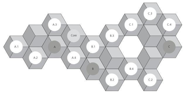
Core = Empty tile with BeoSound Core A, B, C = Amplifier tiles Note: A= Primary amplifier (connected to the BeoSound Core) and B, C= Secondary amplifiers. A.1, A.2, A.3, A.4, B.1, B.2, B.3, B.4, C.1, C.2, C.3, C.4 = Speaker tiles.
