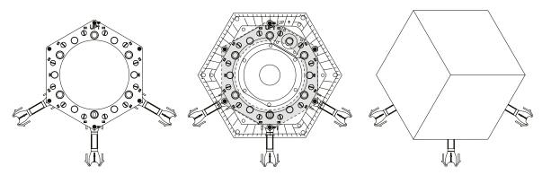
Lay all the star rails down on the floor in the chosen pattern according to the PDF document presented in the Configuration tool. Connect all the star rails with the connection rails.
