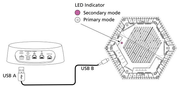
To load the standard filter into the amplifier tile, the tile has to be converted to primary mode. Follow these steps:
