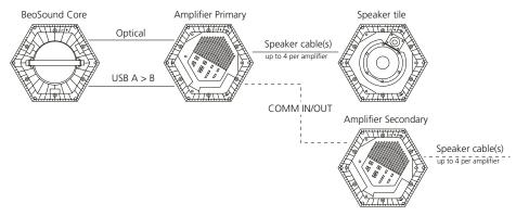
When the filters are applied, and all speakers are tested, you can now disconnect the USB and Optical cable, and replace them with a Power Link cable from the BeoSound Moment instead. If the BeoSound Shape is not mentioned in the speaker menu, use BeoLab 17.
