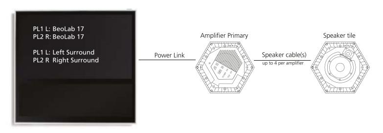
Note: In this example the BeoSound Shape is used as rear speakers in a TV setup.
