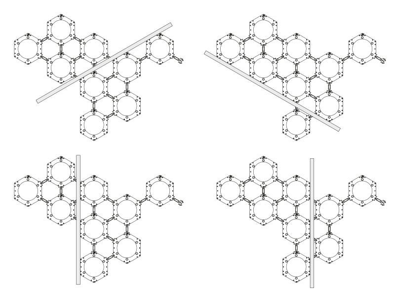
When more star rails are mounted, use a aluminium straight edge tool or a spirit level to level out the star rails crosswise and vertically.
