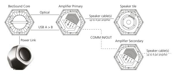
Gain adjustment on BeoLab 19 must be adjusted depending on the number of speakers connected in the setup. Adjust until the bass level is as desired.
