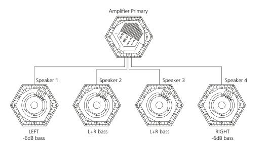
After the amplifier tile has been updated to Primary mode and the standard sound filter has been loaded, the output channels will look like this:
