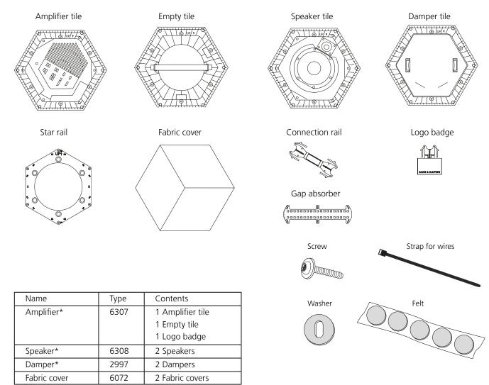
\* Also includes: 2 star rails, 4 connection rails, 4 gap absorbers, 5 felt stickers, 2 straps for wires, 12 PT3x18 torx 10 zink screws, 12 washers
